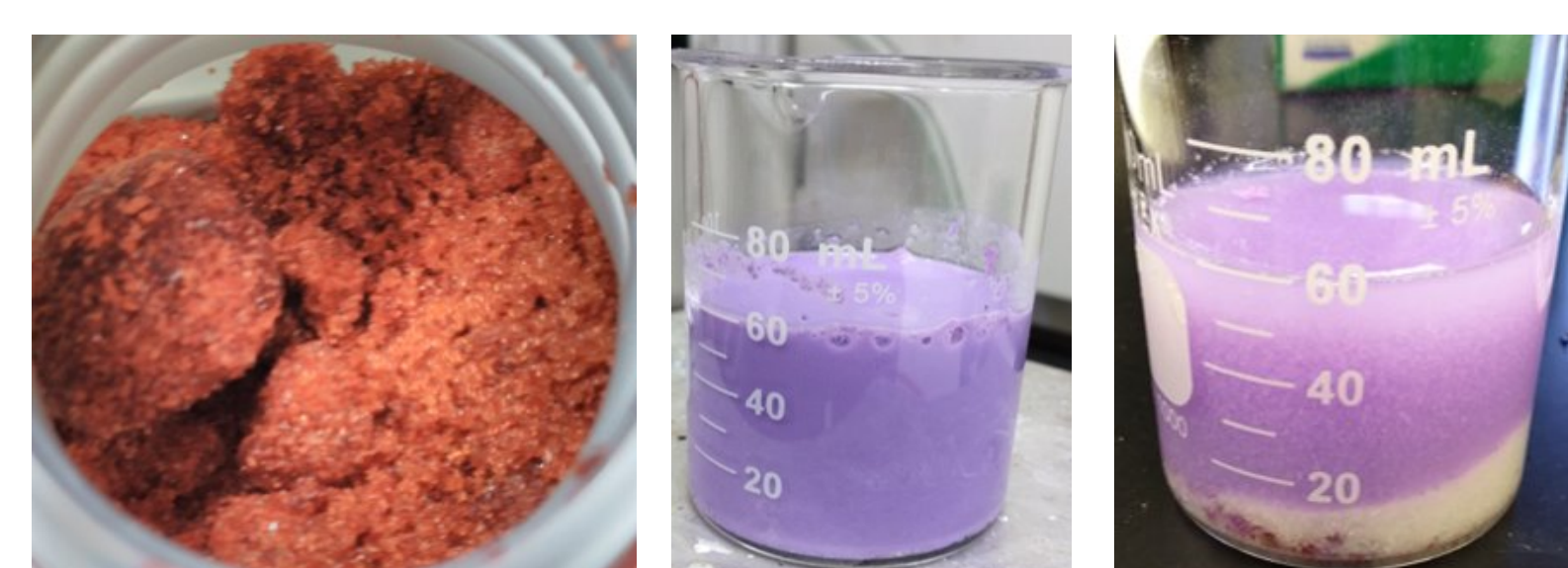
Figure 4. Starting materials for the Co_4PW_9 POM synthesis. Cobalt(II) nitrate hexahydrate (left), sodium phosphate dibasic heptahydrate (middle) and sodium tungstate dihydrate (right).
