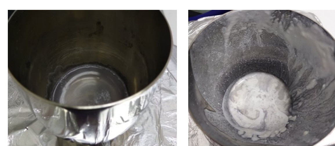
Figure 8. Starting materials for the Nb_6O_{19} POM synthesis. Molten potassium hydroxide (left) and niobium(V) oxide (right)
